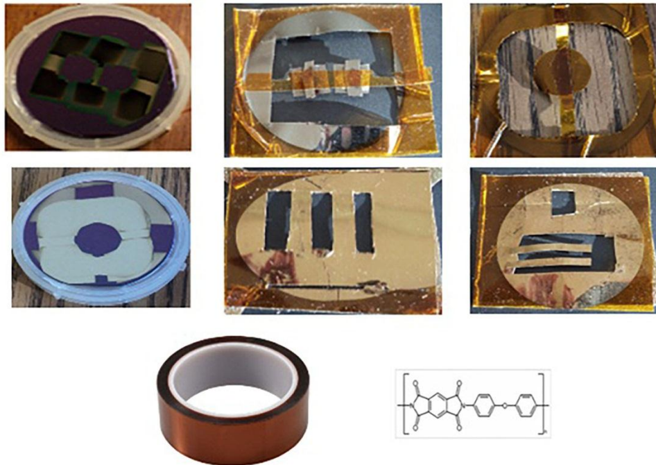
Figure 3.12 Various shadow masking designs made out of polyimide Kapton tape.
